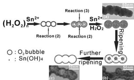
Figure 3. Schematic illustration of the evolution mechanism of intestine-like \text{SnO}_2 . (a), (b), and (c) are the TEM images of the samples obtained after 1, 12, and 24 h, respectively.
